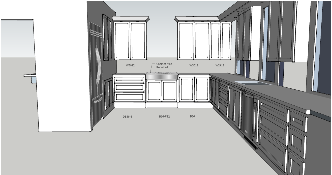
West side kitchen cabinets with 36" Bertazzoni gas stove (requires 6 1/2 " cutout from top of base cabinet).
