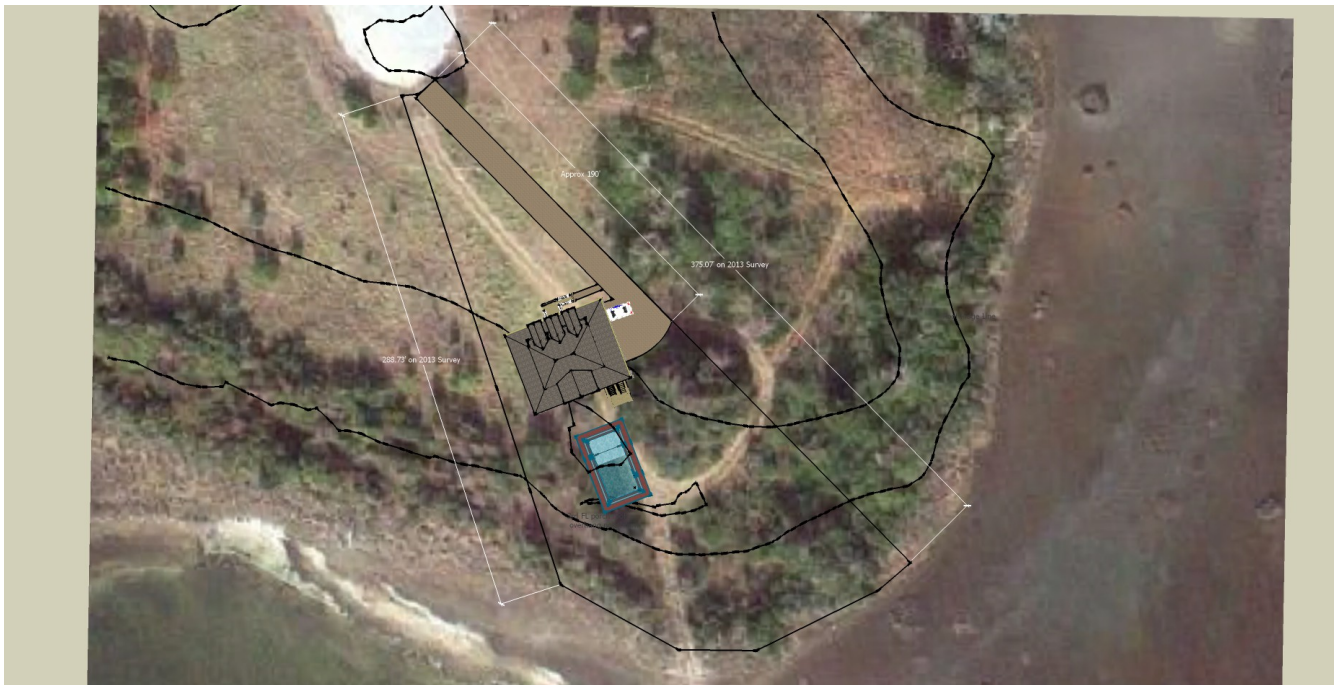
Aerial view showing lot boundary and 2 ft. topographic contour lines overlaid on Google Earth imagery. The house straddles the 8 ft. contour line.
